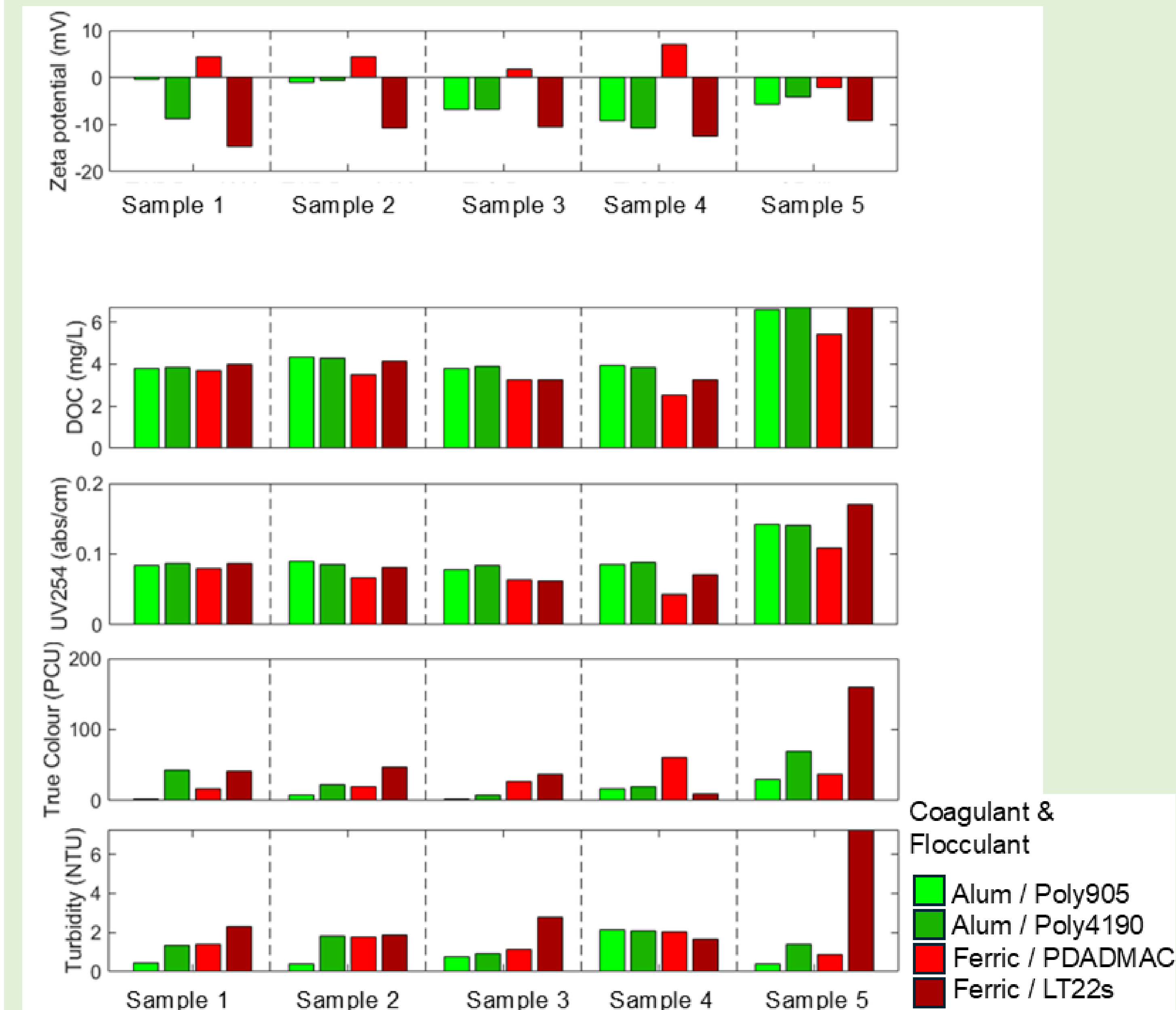
Figure 3: Coagulation-flocculation jar tests results for zeta potential, DOC, UV254, true colour, and turbidity for all other raw water samples.
